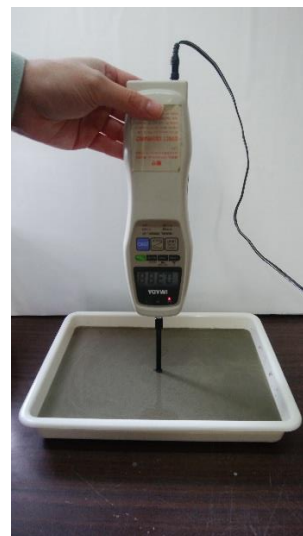
Fig.4 Simple penetration test
