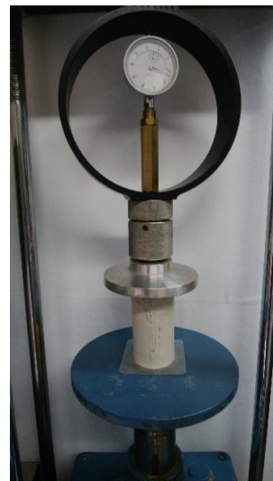
Fig.3 Uniaxial compression test
